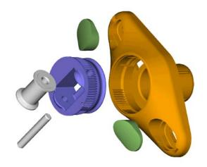
The insert part of the housing (coloured blue) can be removed at any time either before installation or after. This feature will allow for the roller to be removed without unscrewing the housing from the wall. The ability to remove the insert would be an advantage for servicing the shutter if for some reason the control tape needs to be changed.
