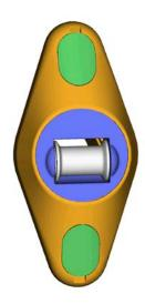
The design criteria was driven by the need for a high quality roller to minimise the wear on the control tape. The roller has retaining flanges either side that will move with the control tape rather then rubbing against it.
