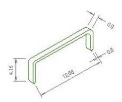
Made from high strength **R316** Stainless Steel that will not corrode and leave ugly stains on the roller shutter.
