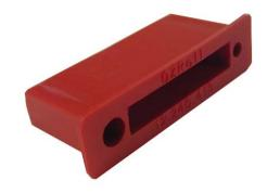
This plastic drill jig is simply inserted into the open face of the guide where it can be easily slid along the length. You then drill the guide through one of the two holes in the jig, maintaining a safe barrier between the drill and guide.
