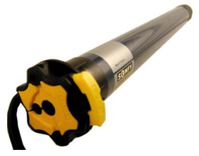
You may be aware that the tubular motor comes in various different sizes. This is due to the large range of shutter sizes. Tubular motors are classed by the lifting capacity, and that is measured in Nm (Newton metres). The most common Somfy LT 240v motors ordered for standard assembled shutters are 10, 15, and 30Nm motors.
