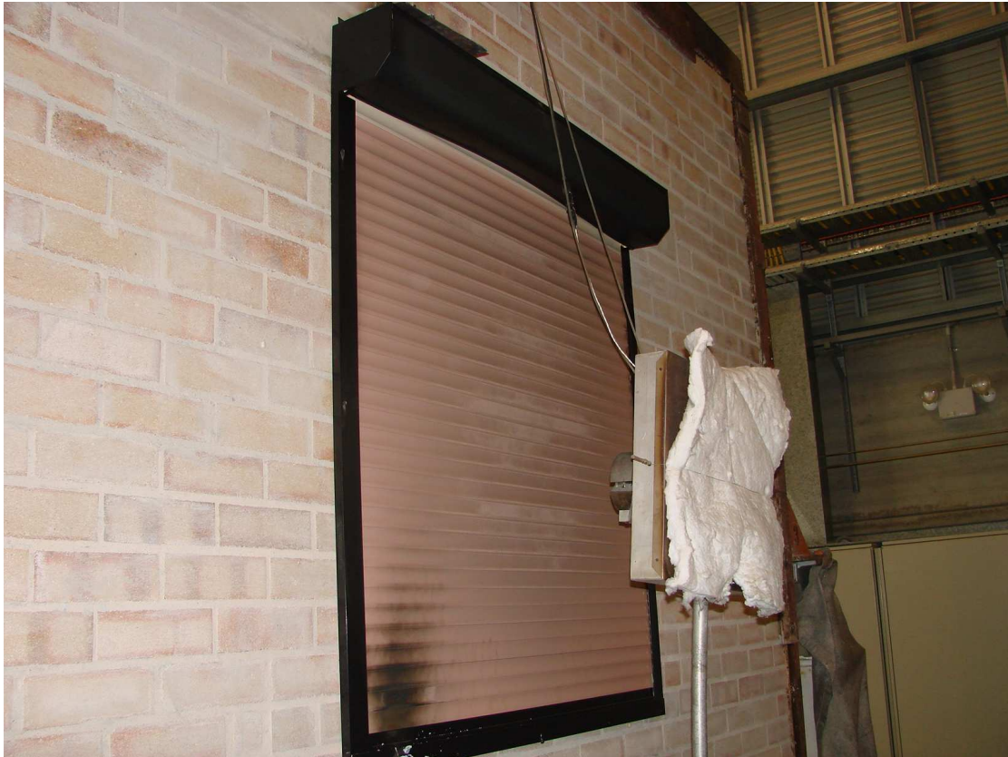
Photograph 5 - Exposed face of the specimen at the completion of testing
