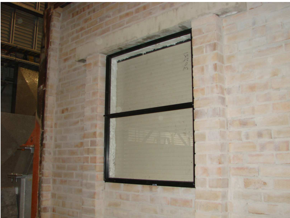
Photograph 2 - Unexposed face of the specimen prior to testing
