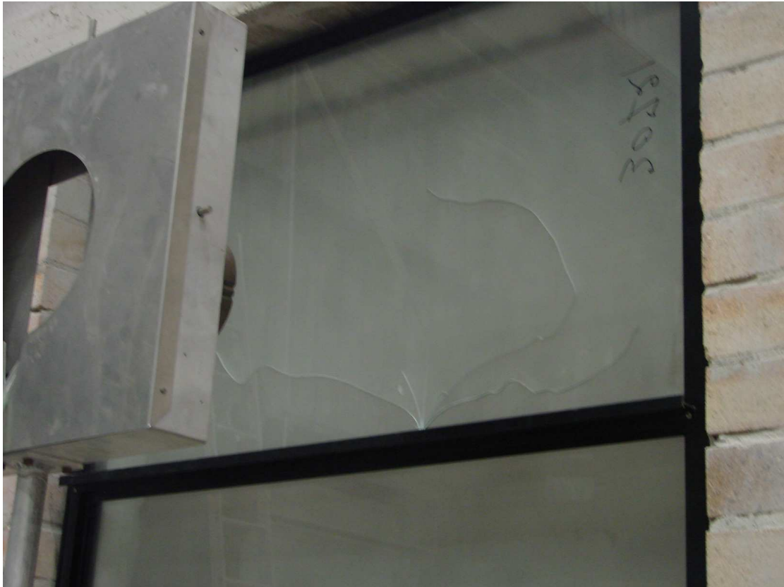
Photograph 4 - Unexposed face of the specimen at 3:15 minutes into the test
