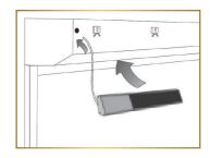
If mounted on the head box or wall it must be in a position that ensures that the E-Solar Pro will receive at least one hour of direct sunlight per day. In these instances the E-Solar Pro should also be installed close to the edge or beside the head box, on the same side as the motor.
