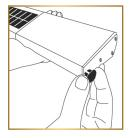
Next, press the stop (i.e. middle) button on the E-Trans transmitter within 60 seconds. When the E-Trans and E-Solar Pro pairing is successful three more clicks will be heard, and the receiver will then leave programming mode.
