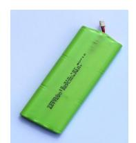
The replacement battery is visibly different to the current battery being supplied with all Controllers and it will need to be fully charged prior to use.
