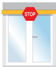
Press Up and then stop the product at the Up limit position. Press the corresponding limit button on the motor until the button springs up.
