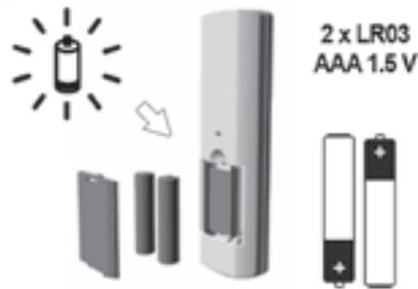
If nothing appears on the screen, remove the battery cover and check the polarity and charge of the batteries.
