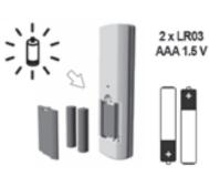
If nothing appeared on the screen, remove the battery cover and check the polarity and charge of the batteries.
